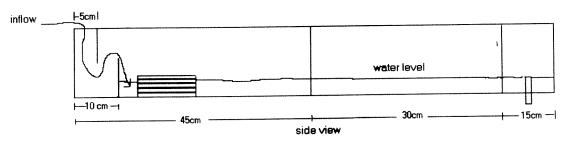
Fig. Diagram of the ammocoete behavioral apparatus.
