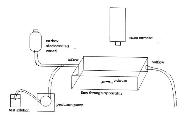
Fig Flow through apparatus and experimental setup.
