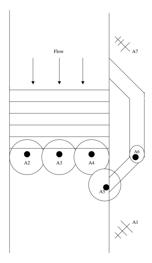
Figure 3. Antenna arrangement at the electrical barrier site in Custer, MI.
