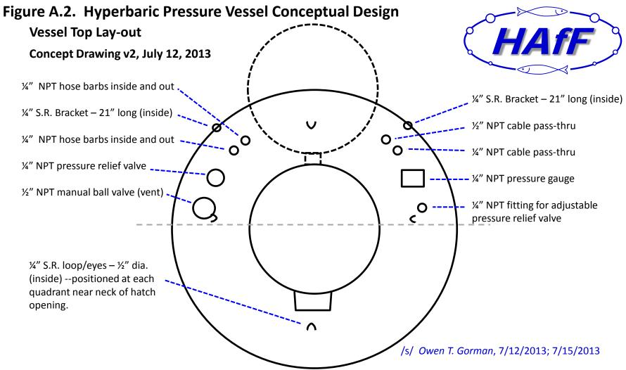
Vessel top: suggested lay-out of connections, pass-thrus, hatch hinge and lift handle
