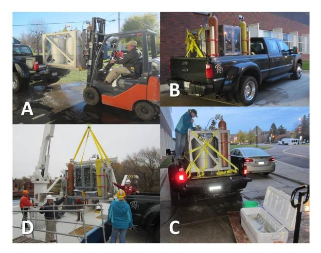
**Figure 2.** Transportability of the Hyperbaric Apparatus for Fish (*HAfF*). A. *HAfF* being loaded onto truck with forklift. B. *HAfF* on truck to deliver fish to the laboratory at University of Minnesota-Duluth. C. Fish being transferred from *HAfF* to coolers at the lab. D. *HAfF* being transferred from R/V Kiyi to truck by crane. Photo credit: Owen Gorman.
