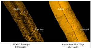
Figure 2. Comparison of sidescan sonar images. North of Painesville Township Park. Water depth: 25ft L-3 Klein: 500 kHz (left) Humminbird :455 kHz (right)
