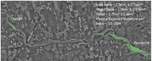
*Figure 10:* Area of exposed shoreline following removal of the main channel weir at average lake level; estimated using SGR DEM (OMNRF 2016), and physical and HEC-RAS model outputs (Annable and Plumb, 2009)
